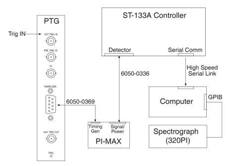
Figure 33. Typical System Cabling
